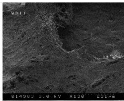
Fig. 6. Dense network of hMSC penetrating the poly-l-lactide scaffold after 21 days of osteogenic differentiation.
